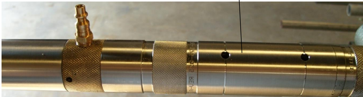
Figure 8: Small Weep Holes
