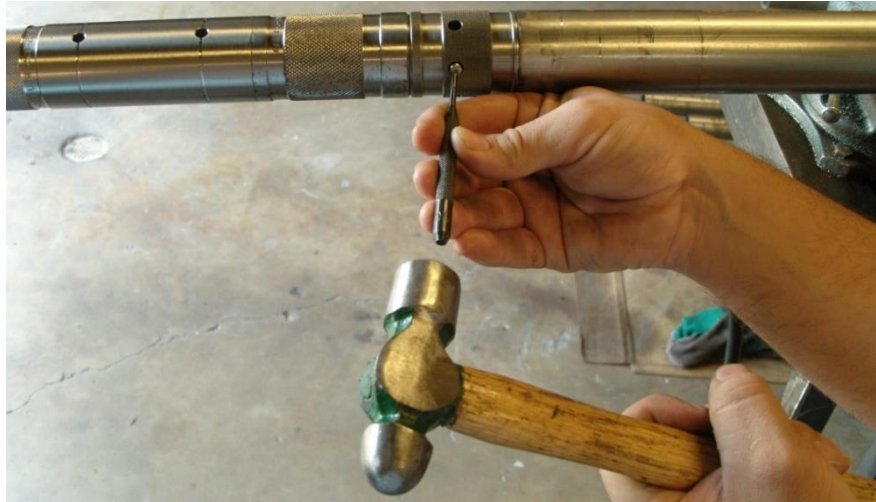
Figure 9: Tapping out Pin on Non-Explosive Neo Thru-Tubing Bridge Plug
