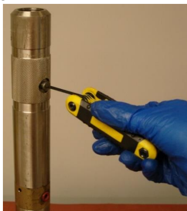
Figure 2: Removal of #2 Parker Plug
