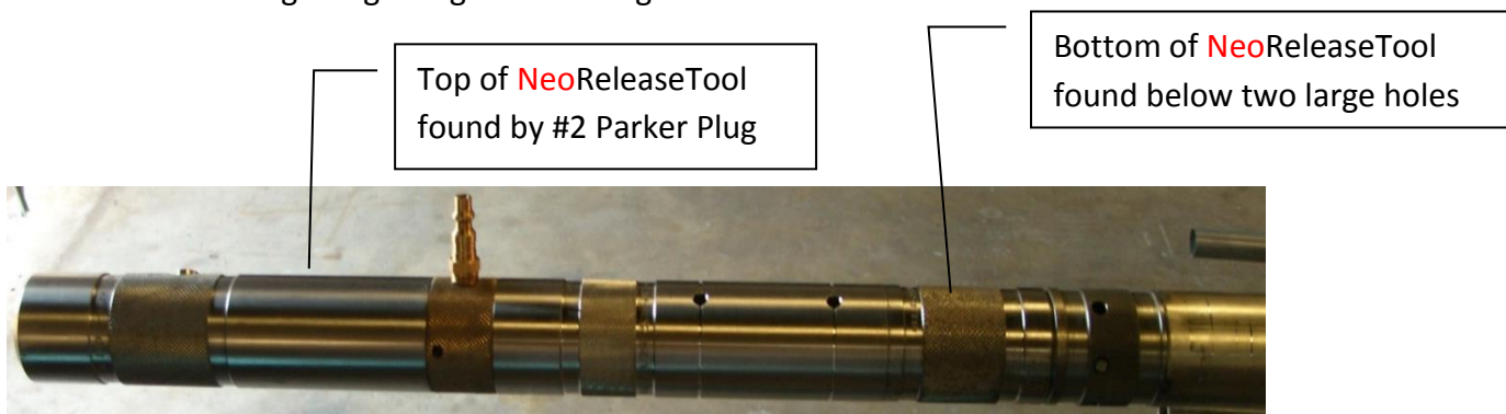
Figure 6: NeoReleaseTool Attached to Non-Explosive Neo Thru-Tubing Bridge Plug
