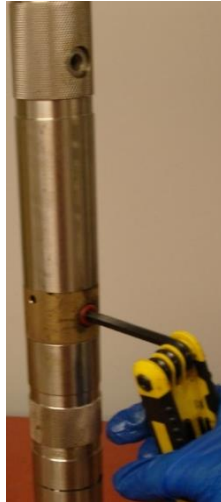
Figure 3: Removal of Pipe Plug
