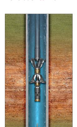
Removable NeoPEPs are thru-tubing mechanical bridge plugs that set in casing and can later be removed from the working wellbore. Standard and NACE MR0175 Compliant Plugs are available.
