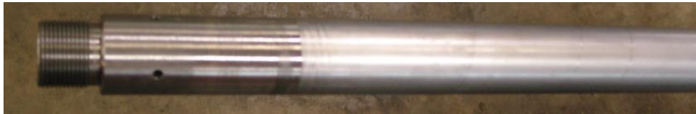
Figure 2: Top Threaded End of NeoT-TBP Sleeve
