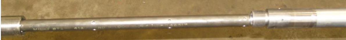
Figure 5: NeoPT being inserted into the NeoT-TBP Sleeve
