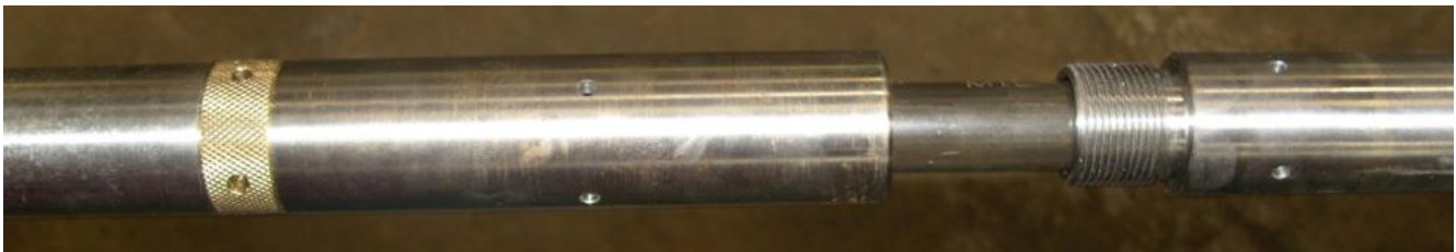
Figure 4: NeoPT being inserted into the NeoT-TBP Sleeve
