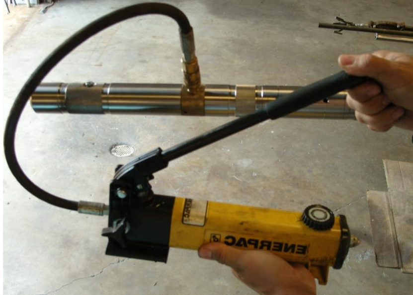
Figure 7: Enerpac Hydraulic Pump Connected to the Pump-in Fixture
