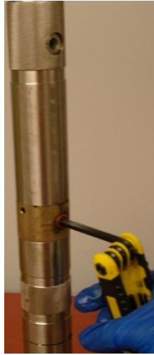
Figure 3: Removal of Pipe Plug
