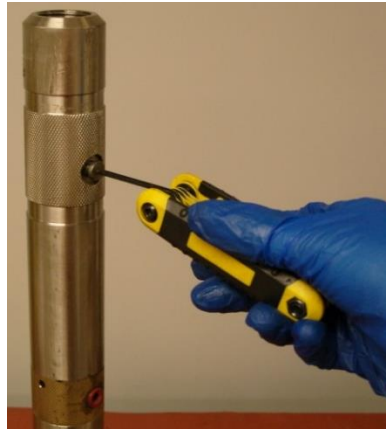
Figure 2: Removal of #2 Parker Plug
