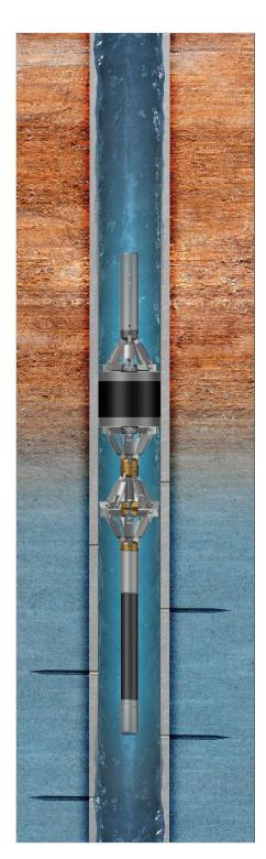
Permanent NeoPEPs are thru-tubing mechanical bridge plugs that pass thru small restrictions and set in casing and openhole diameters up to 3½ times their run-in diameter. Standard and NACE MR0175 Compliant Plugs are available.
