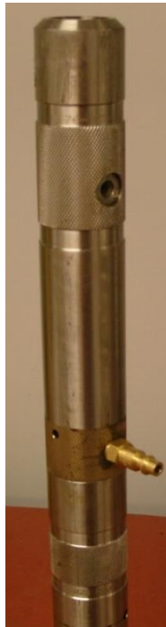
Figure 4: Pump-in Fixture threaded onto Tandem Sub
