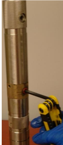
Figure 3: Removal of Pipe Plug
