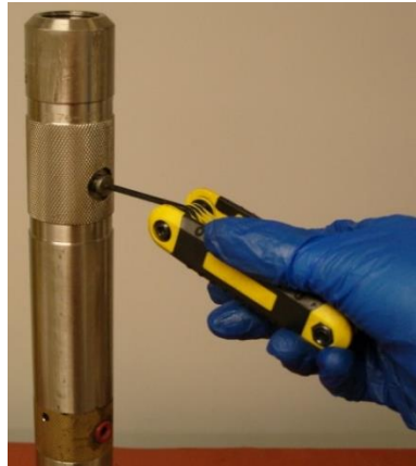
Figure 2: Removal of #2 Parker Plug
