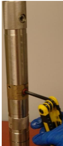
Figure 3: Removal of Pipe Plug
