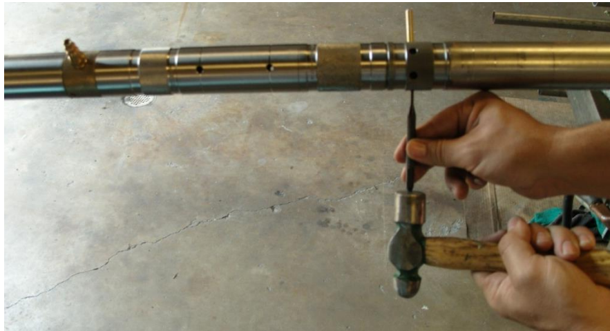
Figure 10: Tapping out Pin on Non-Explosive Neo Thru-Tubing Bridge Plug
