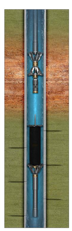
Removable NeoPEPs are thru-tubing mechanical bridge plugs that set in casing and can later be removed from the working wellbore.
