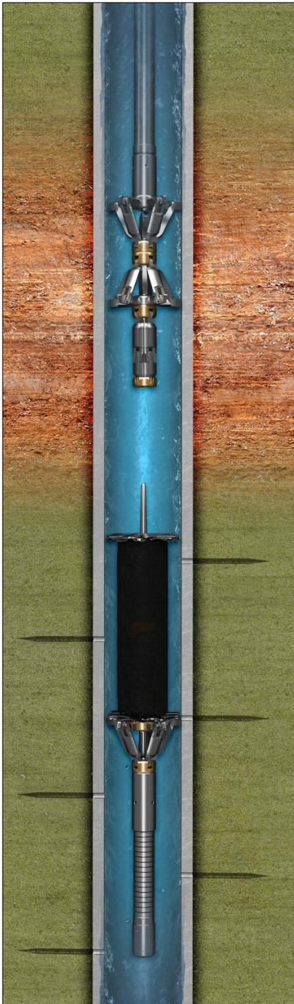
Removable **NeoPEPs** are thru-tubing mechanical bridge plugs that set in casing and can later be removed from the working wellbore. Standard and NACE MR0175 Compliant Plugs are available.
