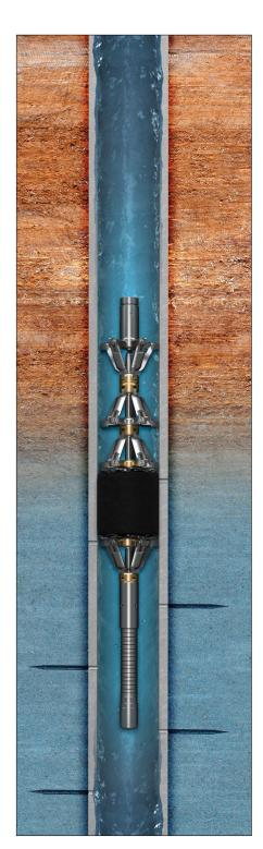
Permanent NeoPEPs are thru-tubing mechanical bridge plugs that pass thru small restrictions and set in casing and openhole diameters up to 3½ times their run-in diameter.
