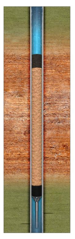
A <u>Permanent NeoPEP</u> combined with a <u>Composite Platform System</u> can provide exceptionally high  $\Delta P$  service from above the plug while providing normal  $\Delta P$  service from below.
