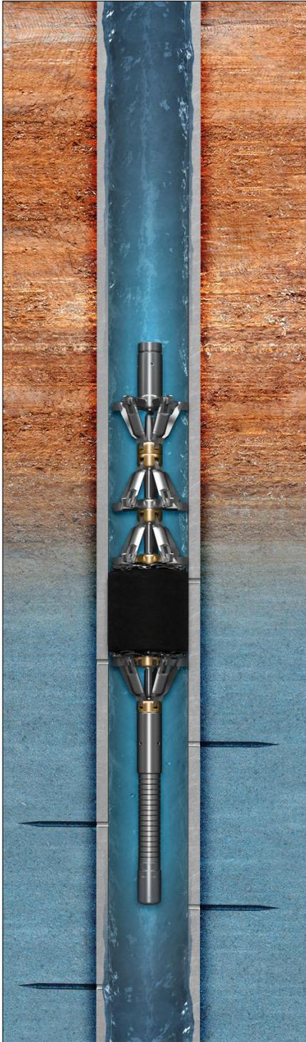
Permanent NeoPEPs are thru-tubing mechanical bridge plugs that pass thru small restrictions and set in casing and openhole diameters up to 3½ times their run-in diameter. Standard and NACE MR0175 Compliant Plugs are available.
